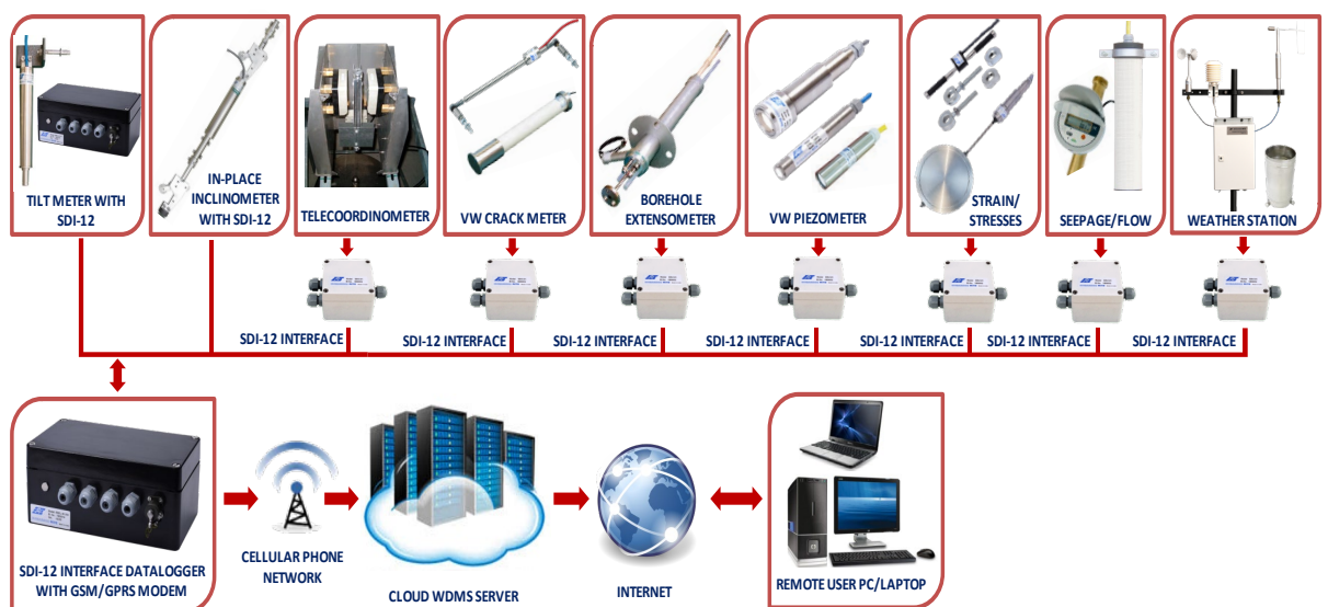
Fig. 5 Dam monitoring instruments on an SDI-12 network
