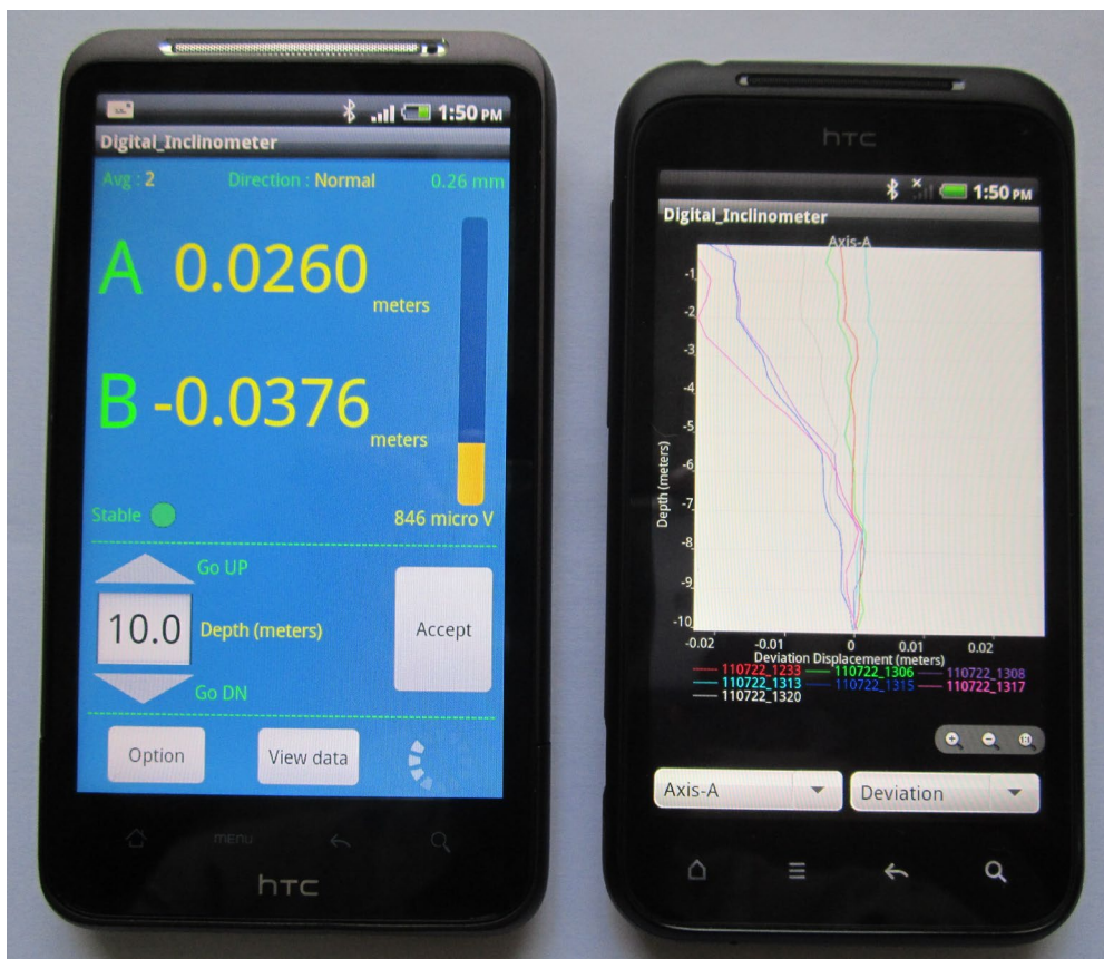
Figure 1: Mobile phones as readout unit (left) and on site analysis of movement profile (right).
