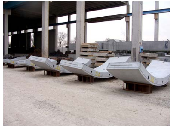
Figure 3.3 Concrete segments with strain gages and pressure cells installed inside
