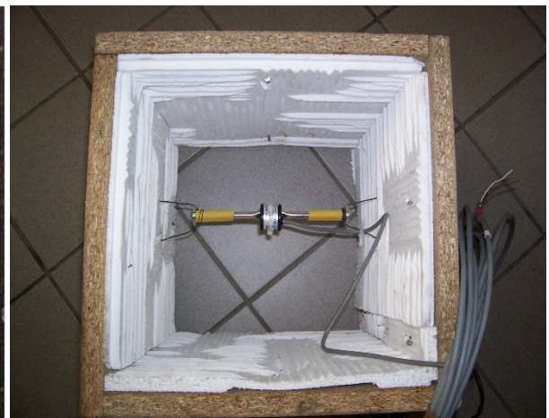
Figure 3.4 Strain gage casted in small concrete blocks for embedment in mass concrete
