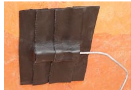
Figure 3.2 Initial thermal protection by insulation tape
