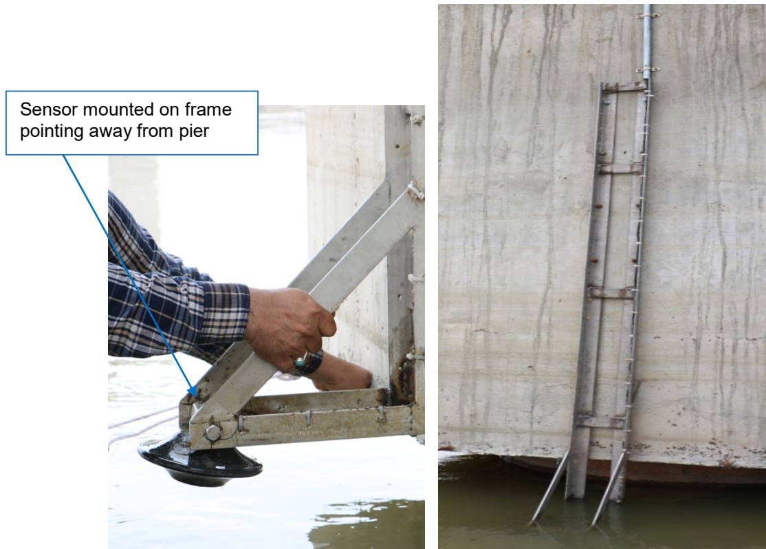
Figure 7: Mounting frame with the sonar sensor fixed on flat surface pier (sensor submerged on water in the right side image)
