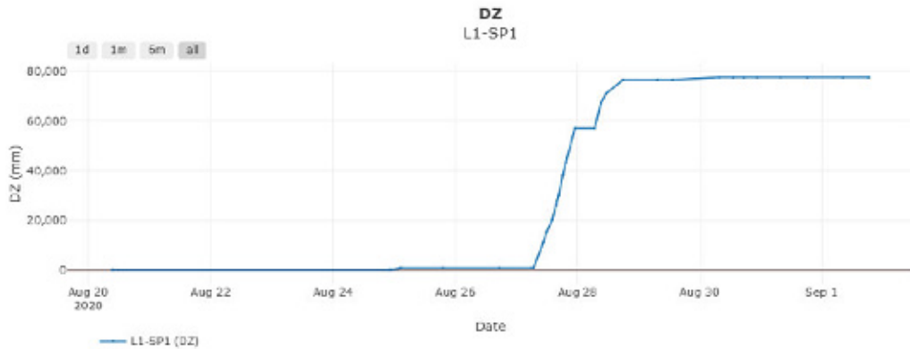
Figure 4 : Graph showing change in elevation of the Link Bridge during its lifting procedure
