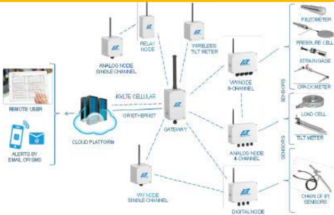
Sensor network with wireless (RF) nodes and gateways
