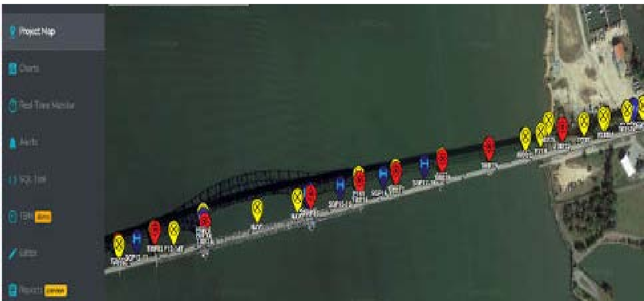
View from the data management software showing location of sensors installed on a bridge
